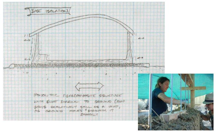
The middle part is the part being tested; the base to attach to the machine is cob reinforced with a box of 6 guage, 6" square mesh, and the top to attach to the loading frame will have a thin bond beam of concrete, held on by all thread attached to wooden blocks in the wall (which is how roof beams are typically attached with this technique)
